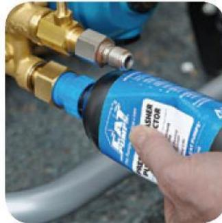
7. Squeeze bottle to inject pump protector fluid into pump.
