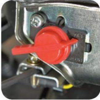
1. Turn engine/motor to Off position.
